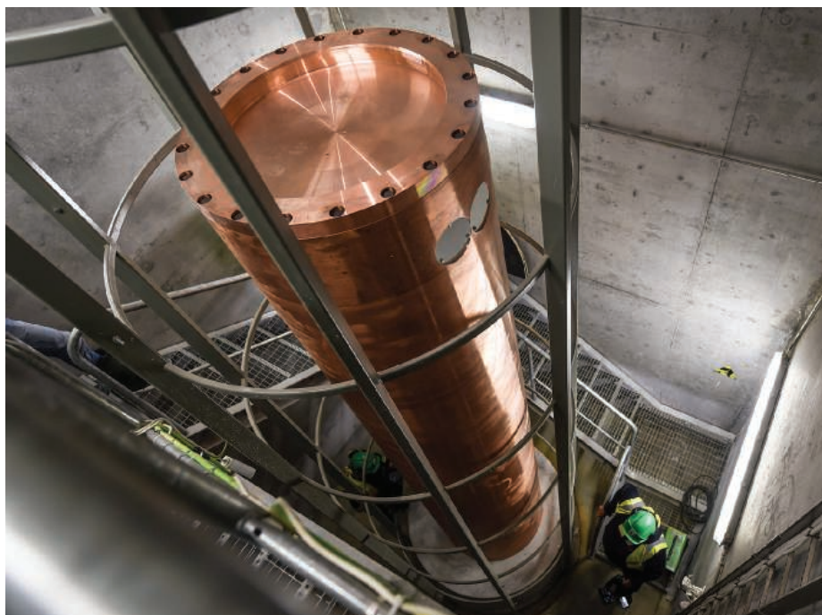
Spent uranium fuel rods will be sealed within thousands of tall, corrosion-resistant copper canisters.
